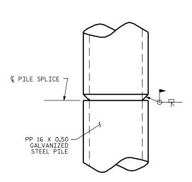
PIPE PILE SPLICE DETAIL
